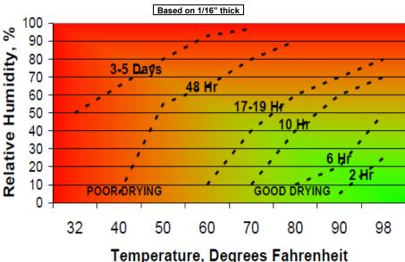
Graph Reference - The color-coded graph provides an easy-to-interpret map of joint compound drying time ranges based on the relative humidity and temperature conditions present on a job. To estimate joint compound drying time, simply select and cross-reference a temperature and relative humidity range to determine approximate drying time per coat (1/16 inch nominal).
